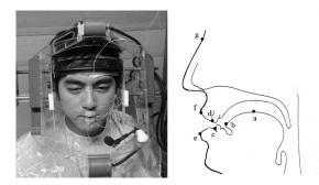
Figure 2. Seven locations of transducer coils. Five articulatory points were (a) the tongue body, (b) the tongue tip, (c) the jaw, (e) the lower lip, (f) the upper lip. In addition, two reference points were used: (d) upper front gum line, (g) the nose bridge which were used to correct for any head movement during the experiment.
